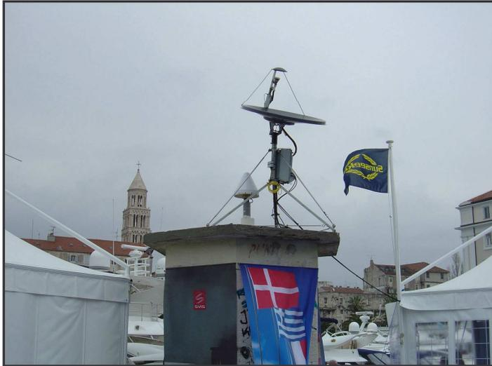
**Figure 4.** CGPS antenna covered by a satellite dish in April 2005.
